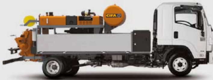
UB504 version mounted on truck
