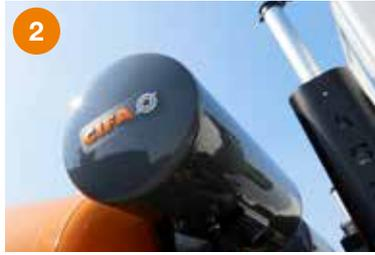
2 Water tank (capacity from 400 to 1200 liters).
