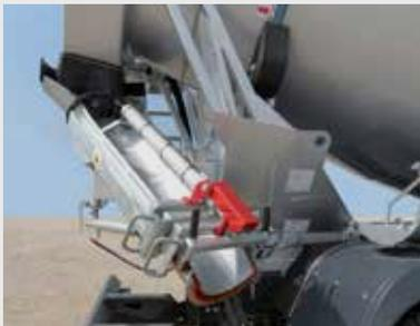
"SL 45" hydraulic extractable discharge chute.
