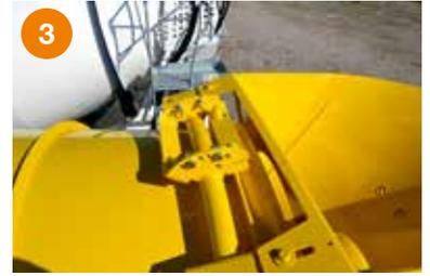
3 Drum anti-rebound system to keep the drum in the right position during the transport phase.
