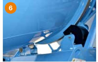
6 Drum rollers. Single or double type according to the truck mixer model.
