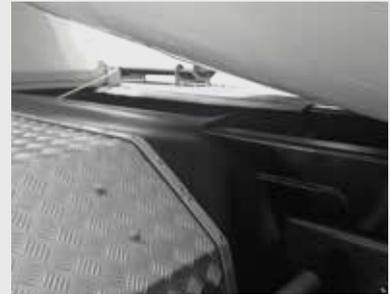
Rubber cover protection between aluminum mudguards and mixer frame.
