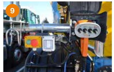
9 Electronic control system. CSD Constant Speed Drive (for CSD version mixer).
