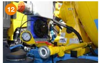
12 Double water inlets. Water can be filled from both right and left side of the truck mixer. Heat exchanger with oil tank. Manometer for concrete consistency.
