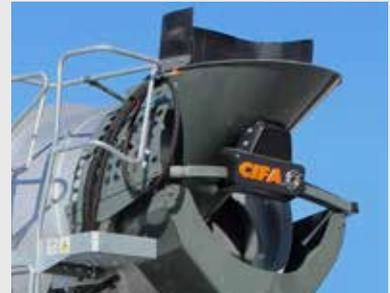
Rubber sleeve on the loading hopper.
