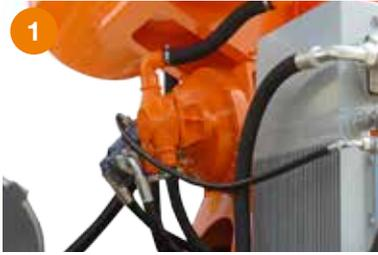
1 Water pump installed on the reducer.
