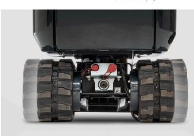
Hydraulic hammer piping is integrated as standard for efficient hammer operation inside buildings.
