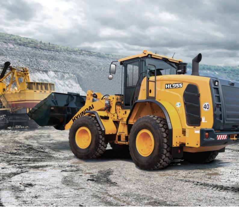
**Net Power** 197 HP (147 kW) / 2,200 rpm **Gross Power** 200 HP (149 kW) / 2,200 rpm **Travel Speed** 40 km/hr (24.9 mph) **Operating Weight** 15,100 kg
