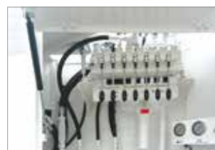
BOOM PROPORTIONAL DISTRIBUTOR Ergonomic hydraulic controls for boom.
