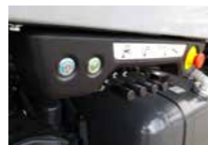
HYDRAULIC OUTRIGGERS CONTROL Hydraulic controls on both sides of truck pump. The machine emergency stop is also positioned nearby.
