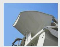
Loading hopper with rear straight side shape.
