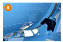
Drum rollers. Single or double type according to the truck mixer model.
