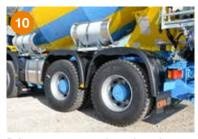
Polymer rear mono-axle mudguards. Double-axle mudguards made of aluminum are available on demand.
