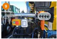
Electronic control system. CSD Constant Speed Drive (for CSD version mixer).
