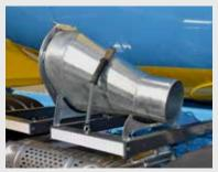
Cone shaped chute with end diameter 200 mm.
