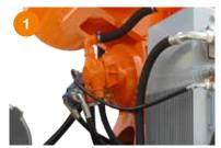
Water pump installed on the reducer.
