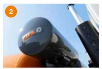
Water tank (capacity from 400 to 1200 liters).
