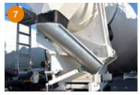
Hot galvanized discharge chute. One-piece type, lenght 1200 mm.
