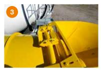
Drum anti-reboud system to keep the drum in the right position during the transport phase.
