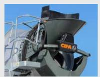
Rubber sleeve on the loading hopper.
