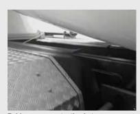
Rubber cover protection between aluminum mudguards and mixer frame.
