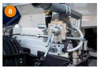
Manual control system driven by flexible cables (for Basic version mixer).
