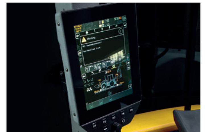
RCI alerts the operator and halts the backhoe in the event of a tipping risk.
