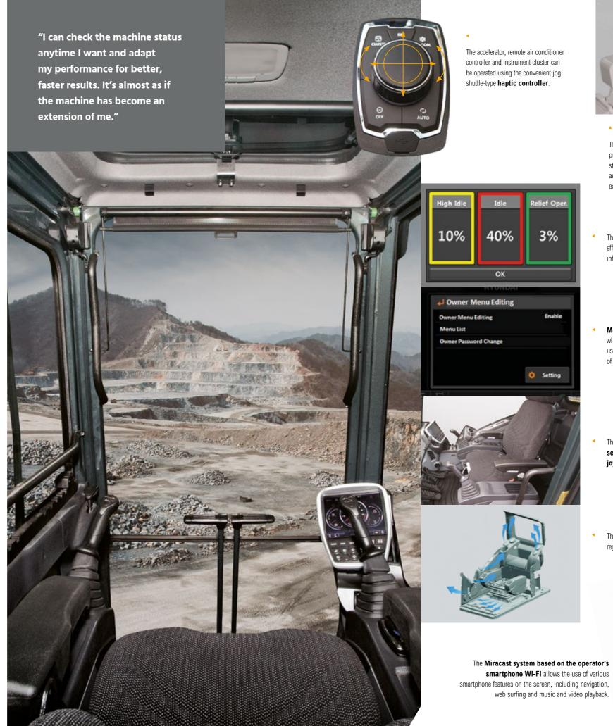
The instrument panel is optimised to provide quick, easy access to machine status information as you work. It features an 8-inch touchscreen monitor for excellent legibility.
