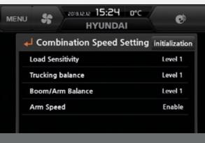
"The control technologies are well thought-out and save me time and money on every job." The combination speed setting system allows operators to balance load sensitivity and boom priority against arm and swing. Select from five levels of load sensitivity to adjust initial flow rate for boom-up and arm-in operation according to attachment weight. Ten levels of boom priority can be selected to balance boom operation against arm and swing.
