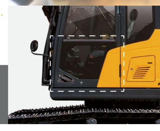
The **auto safety lock** feature prevents unintentional ignition. While the auto safety lock is activated, the excavator is not controlled by the RCV lever.
