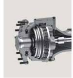
The **brake discs** are manufactured using a durable sinter material to suppress generation of heat and vibration. They extend the lifetime of the brakes, while also integrating a service-friendly design.
