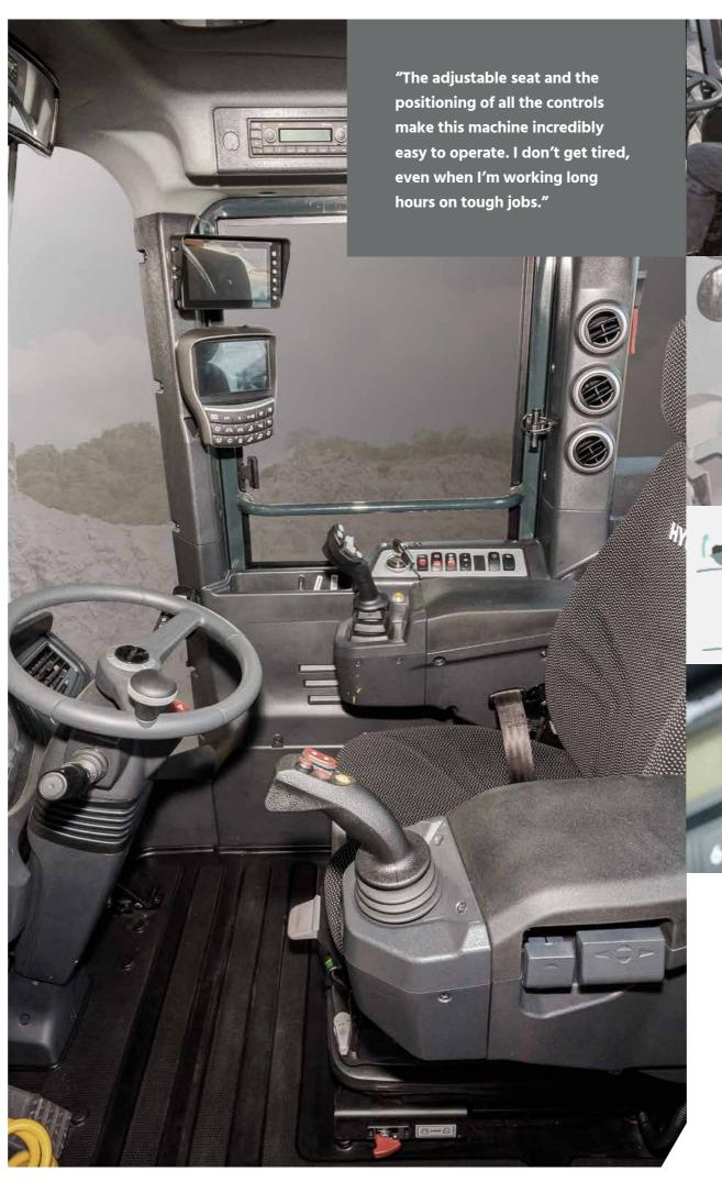
The HL940A has a large, comfortable seat with a headrest and fully adjustable armrests. Cabin space is increased by integrating the attachment control levers in the armrest, which also makes operation more comfortable. An air suspension seat and seat heating are available as options.
