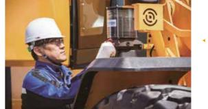
Uptime has been increased by extending the standard service interval for the oil and oil filter to 500 hours, which also reduces maintenance costs, and by adding an optional autogrease system.
