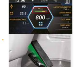
This option ensures that the engine shuts down automatically when the machine is at rest to cut fuel consumption and prevent unnecessary emissions.
