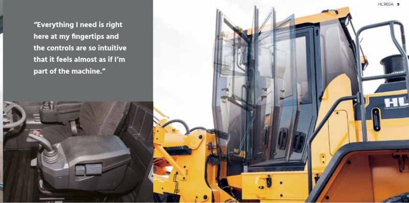
The HL960A has a large comfortable seat with heating as standard. The seat and armrest are fully adjustable and, for added comfort, an air suspension version is available as an option. Thanks to the electro-hydraulic implement control lever, less force is needed to operate attachments, helping you to work longer and more productively.
