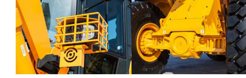
**Axle seal guards** are bolted to the axle shaft to prevent materials (such as metal springs or wire) from cutting and damaging the axle seals when the wheels are in motion.
