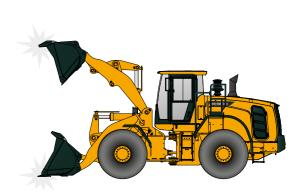
The soft end stop function reduces the hydraulic speed of the cylinder as it reaches the end of its stroke. This lessens the shock load of the stroke for increased operating comfort and better material retention.
