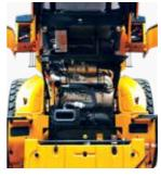
With the optional **auto greasing system**, grease is applied to lubrication points automatically when needed. The correct dosing is ensured and lubricant is applied uniformly, reducing grease consumption and eliminating waste. The **tilt-back engine hood is fully retractable** and can be **opened electrically** for easy access to the sealed engine room and cooling room. The engine room is designed to prevent the possibility of fire caused by the inflow of foreign materials.
